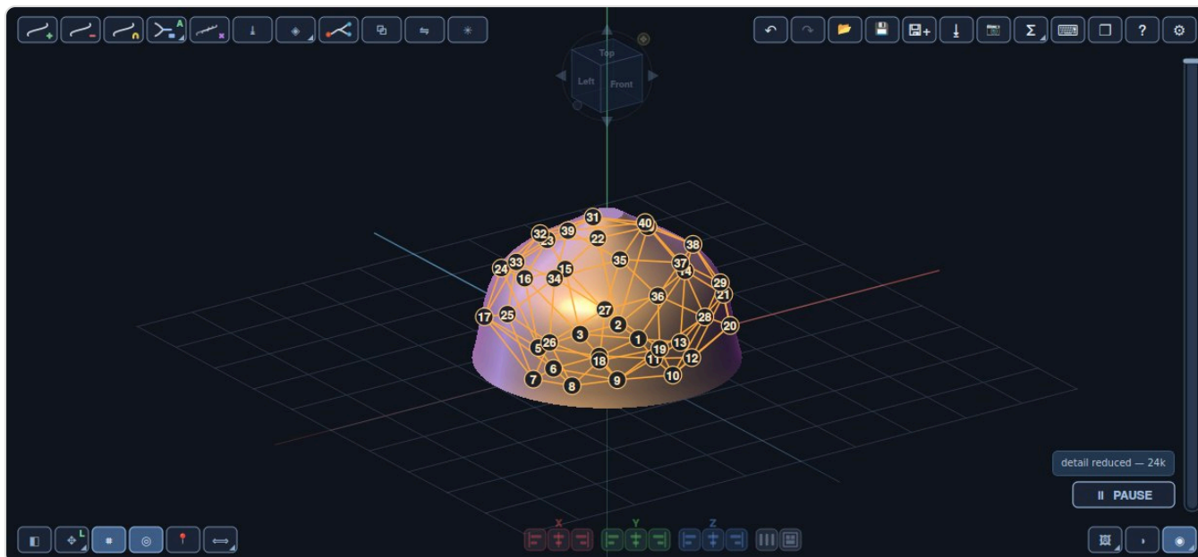
A dome as a near-equal strut net, its nodes numbered.
